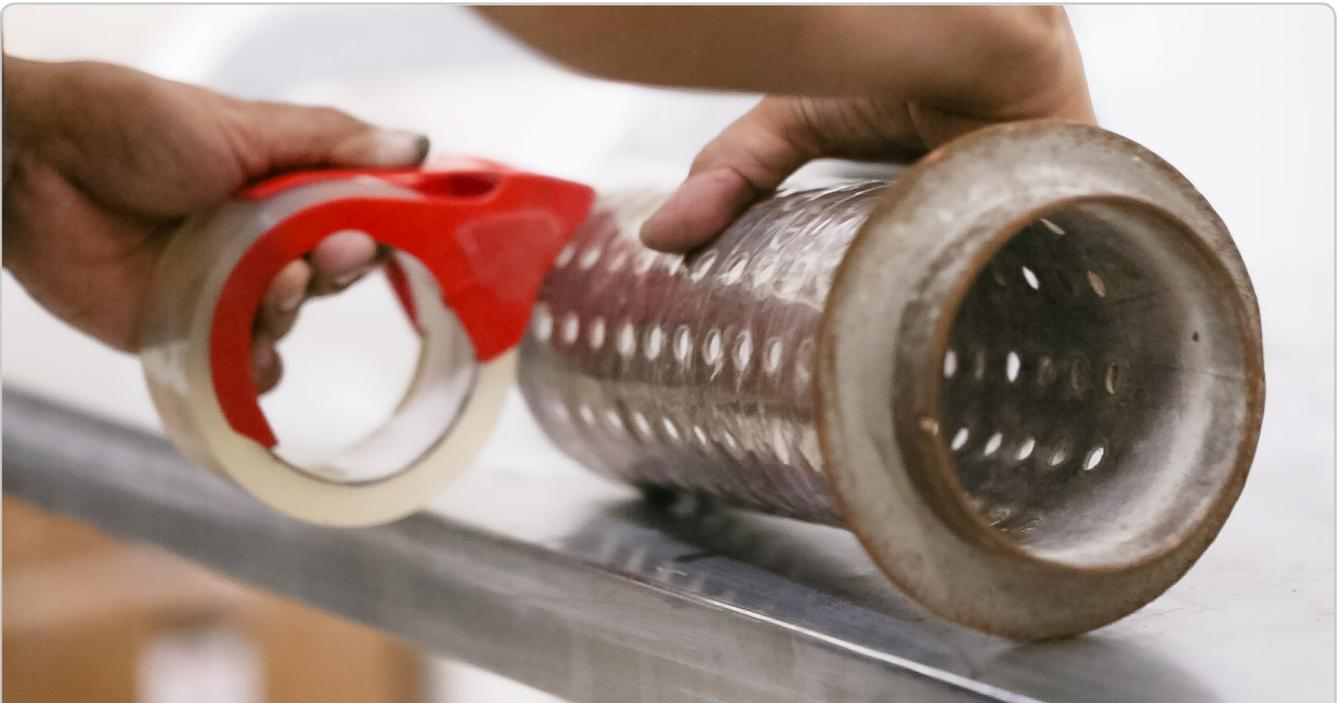
Attach a casting flask to the sprue base. If the flask is perforated, wrap it with clear packing tape to contain the investment.
