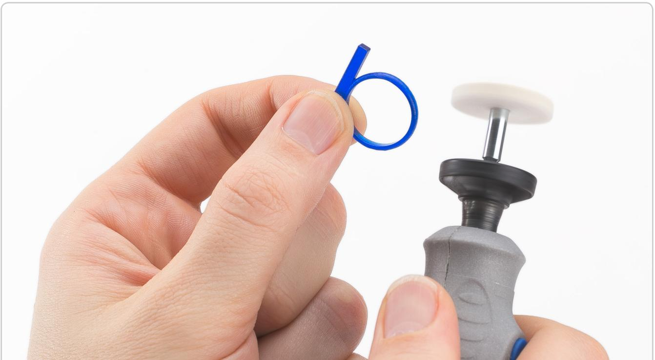
Polish the surface using polishing paper or a rotary tool with a buffing attachment.
