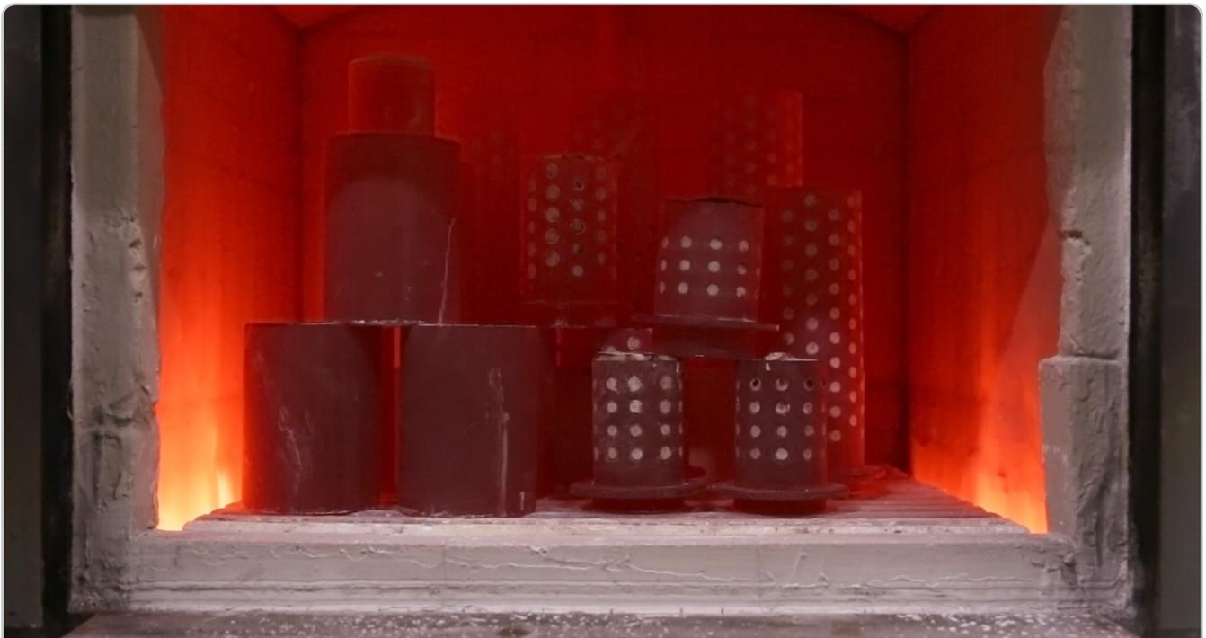
Place the casting flask in a cold furnace and heat according to the burnout schedule provided on page 2. Remove the mold from the furnace and cast metal.
