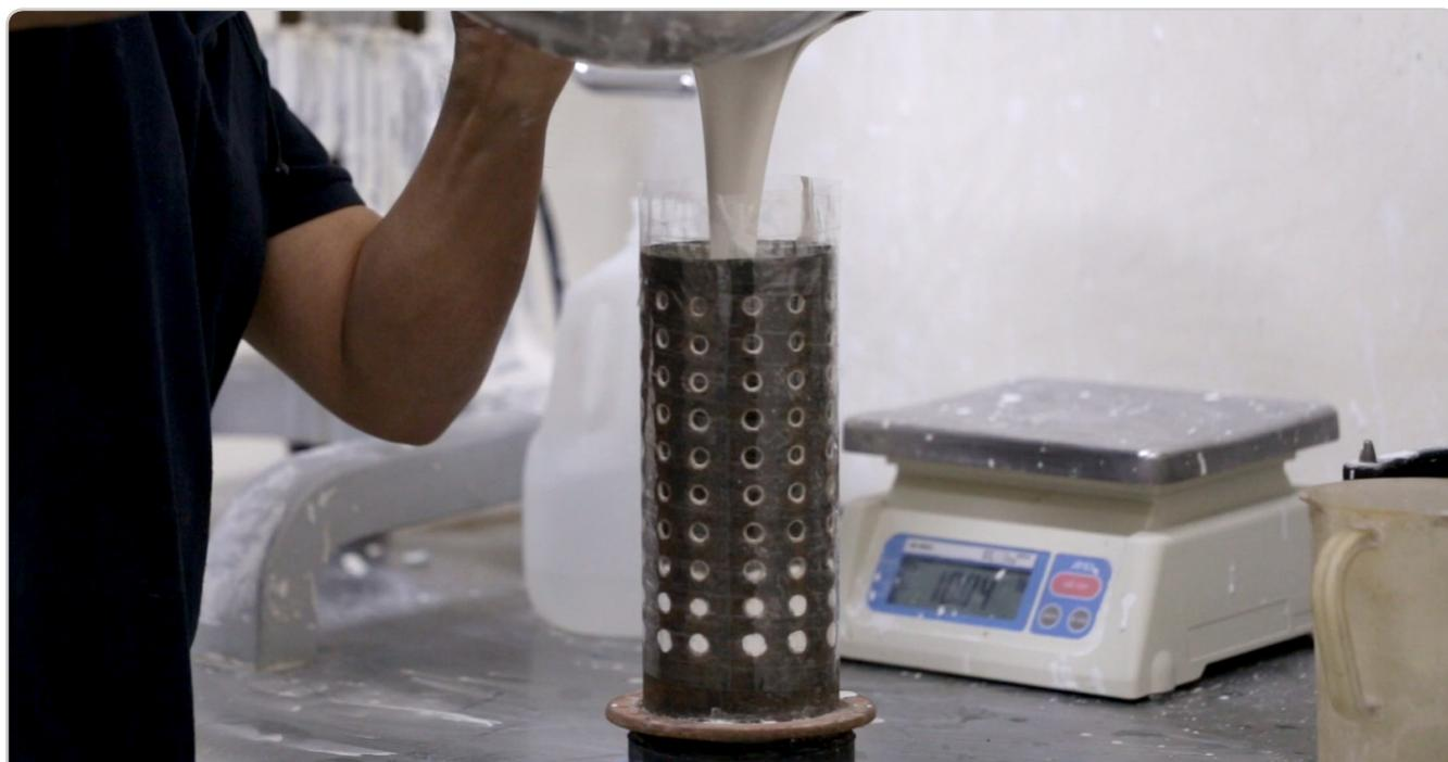
Slowly pour the investment into the casting flask. Pour the investment down the side of the flask to avoid damaging the fragile wax tree.
