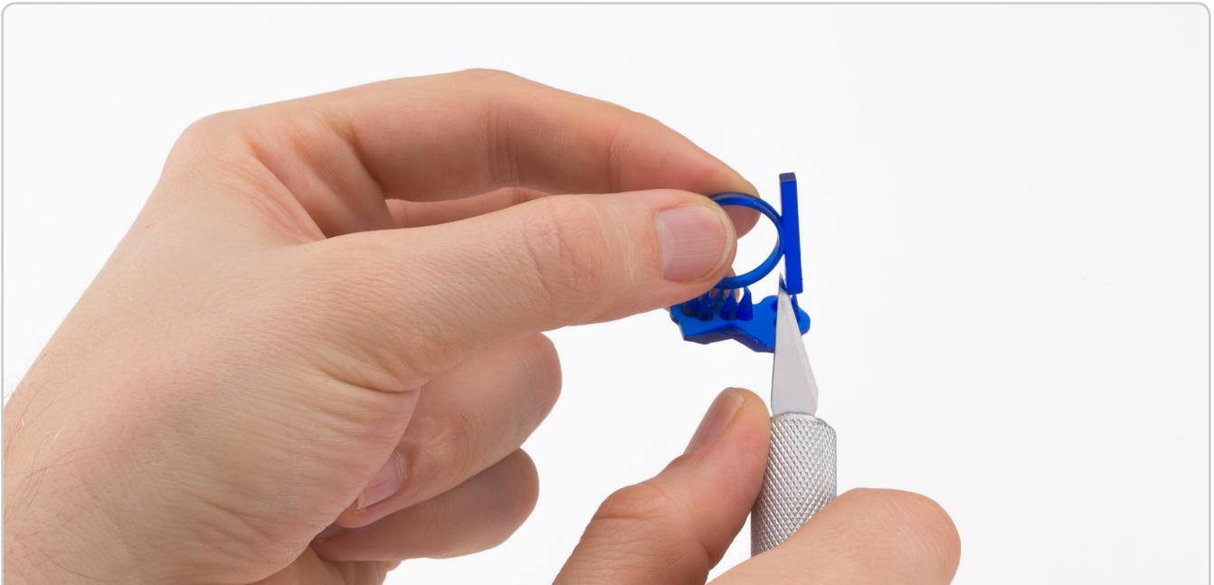
If necessary, carefully remove support material from your print. Using fine sandpaper (400 grit and above), gently sand away support marks.
