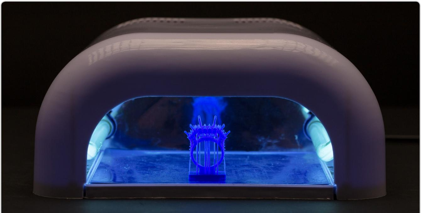
Cure the part under UV light until the surface is hard and rigid. Discoloration of the part is normal during this process.
